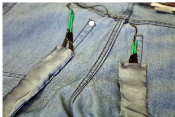
Figure 3: Integration of bend sensors inside jeans
