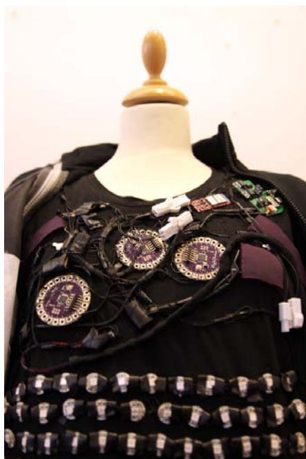
Figure 4: Close-up inside platform (sweater): screen, electronics and sensors.
